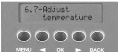
This function can be used for precise adjustment of the internal temperature sensor. It is first necessary to obtain the exact temperature inside the gun cabinet (e.g. by leaving a thermometer inside the gun cabinet for at least an hour).
