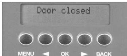
**N.B.:** *if the batteries are low, the "Door closed" message will be followed by the message "Battery low! Change battery."*
