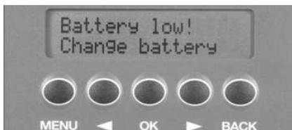
In this condition, in order to save further consumption of the nearly flat batteries, the blue backlighting of the display will not be activated until the batteries are changed.
