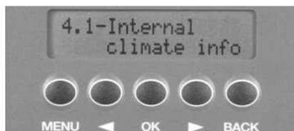
This menu can be used to display the temperature and humidity inside the cabinet. Press **OK**; the data will be displayed as in the following example:
