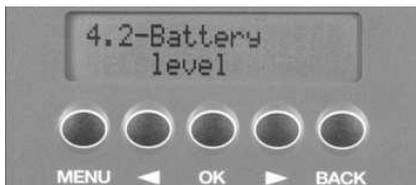
This function can be used to check the battery level. This information is shown as a percentage, followed by an estimate of the number of days remaining before they need to be changed. This calculation is made (starting 30 days after insertion of the batteries) on the basis of how much the cabinet has been used up to that point, and therefore depends on how often the door has been opened/closed.
