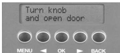
turn the knob one quarter of a turn in a clockwise direction and open the door.
