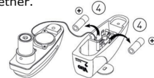
Replace old batteries with 2 new ones (12V type MN21). Close the disc lock again, paying attention not to crush the wires.
